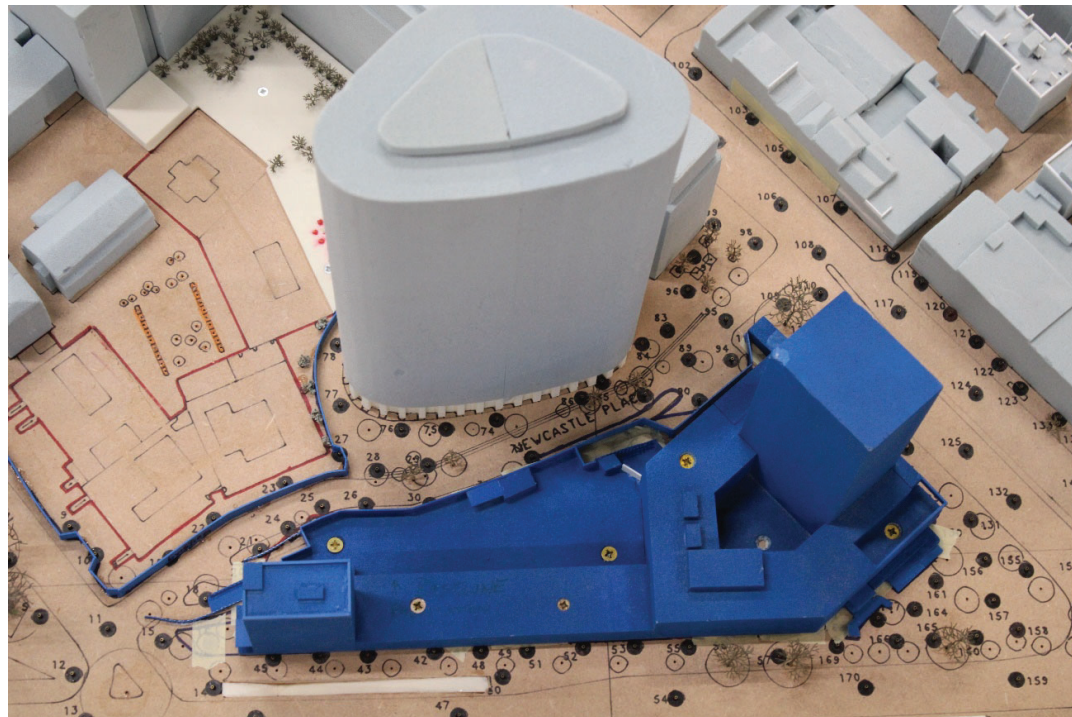
Figure 3: Configuration 1 - view in the Wind Tunnel from the south
